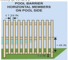
6. Where the barrier is composed of horizontal and vertical members and the distance between the tops of the horizontal members is 45 inches or more (1143 mm), spacing between vertical members shall not
